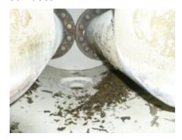
In addition to this, it was noted that the cylinder has previously been shot blasted and lined with a corrosion proof paint. As this would not survive the acid descaling process the loose material was removed manually and the surfaces carefully scoured.
